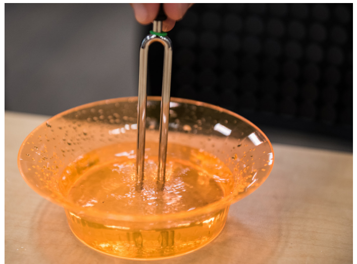
A tuning fork transfers its vibrational energy to the water surrounding it causing small ripples.
